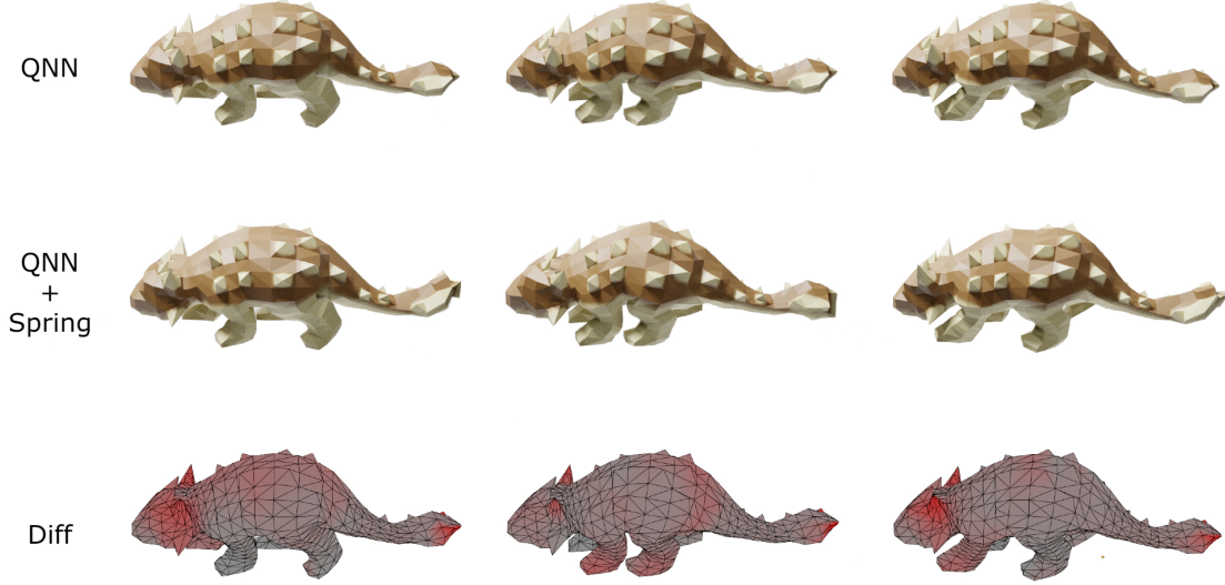
Figure 2.6: Secondary dynamics are added to a low-poly ankylosaurus. Notice how the zero-restlength springs (second row) manage to add dynamic motions on top of quasistatic result (first row), especially around the ears, tail, and back region.
